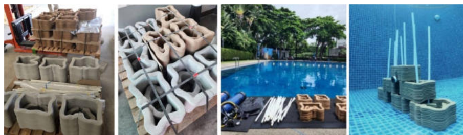
Fig. 13 logistic / transportation process (left), sustainable logistics (left center), testing operation of 3DMARs in pool (right center), triangular arranged format underwater (right), Image courtesy of Torpong Limlunjakorn
