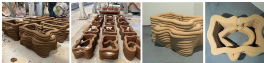
Fig. 12 3DMARs prototyped and manufactured at SCG factory (left, left center), Isometric view of 3DMARs (right center), Top view of 3DMARs (right), Image courtesy of Torpong Limlunjakorn
