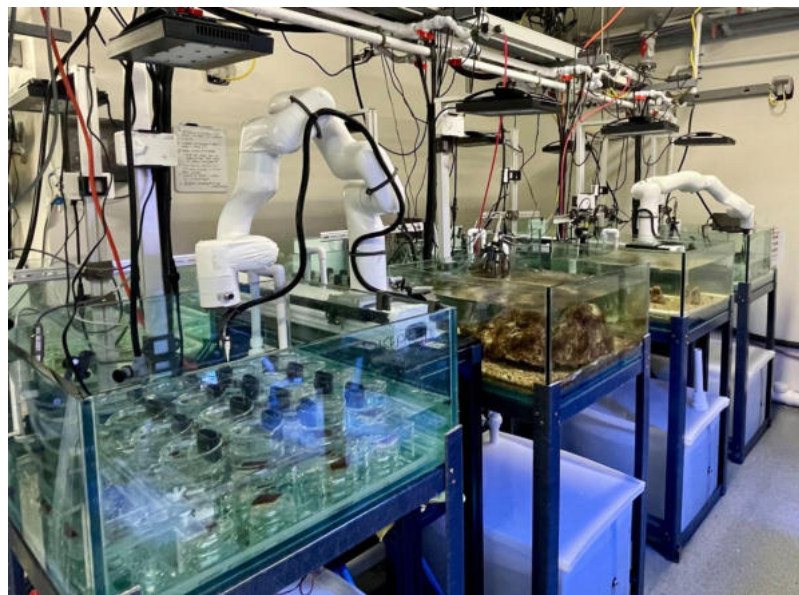
Fig. 1. Panoramic view of the STAR system. The picture shows the two robot arms dosing the experimental corals with artificial seawater (previously exposed to healthy or diseased coral colonies) and ammonium.
