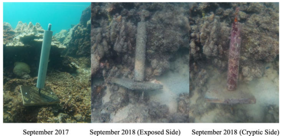
Fig. 3 CaCO 3 production by secondary carbonate producers over a 1-year period on PVC pipes deployed at Nearshore (Fasht Al Adhm). NB: exposed=high light, cryptic=low light
